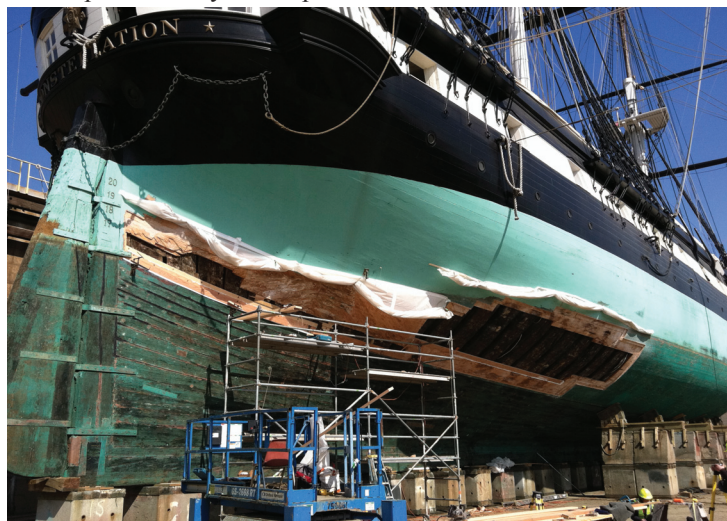
Detail showing the large area of deterioration in CONSTELLATION'S laminated hull planking. The darker areas are the original frames. Shipwrights used the scissor lifts and scaffolding to access the work areas, some of which was over 30 feet above the floor of the dry dock.
