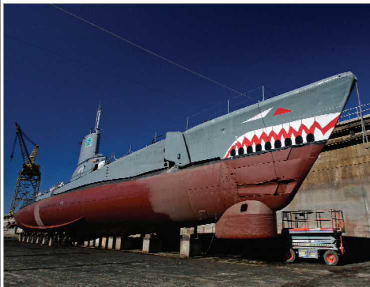
USS TORSK in Dry Dock with Partial First Coat of Epoxy Paint Photo Courtesy of Doug Schmenner
