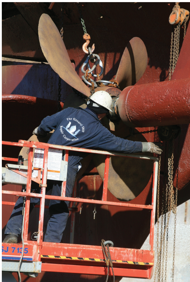
The Starboard Propeller of USS TORSK Being Removed. The Port Side Propeller Was Removed Before the Boat Came to Baltimore.
