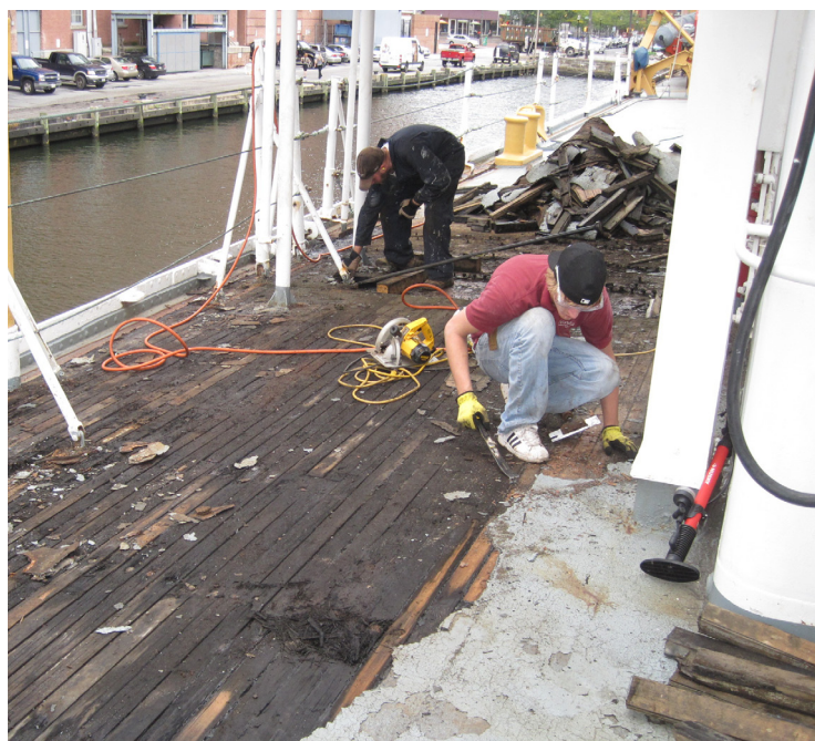
Matt Singleton and Brian Baublitz remove rotten wood and rubber overlay from the deck of USCGC Taney.
