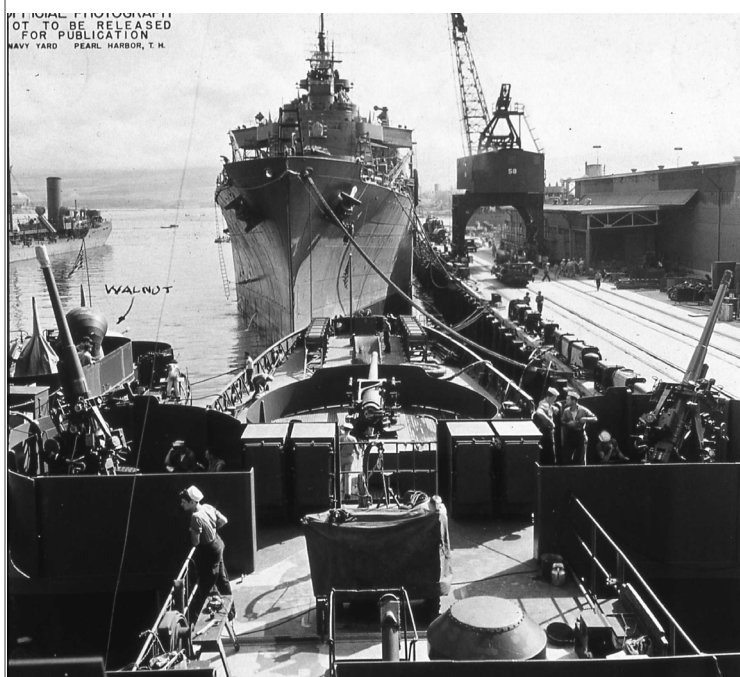
Taney 266 "An early World War II view of TANEY's quarterdeck as seen from the ship's radio room. Note in the foreground the two 3"/50 caliber mounts (port and starboard) which would have been in action against Japanese aircraft on 7 December 1941.
