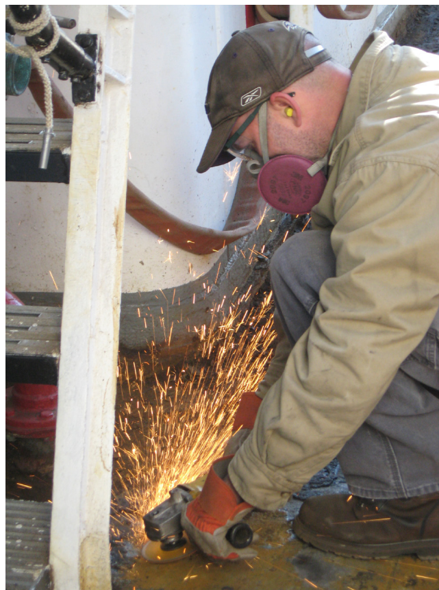
Matt Singleton grinds away years of rust and scale forward, on the port side of USCGC Taney.
