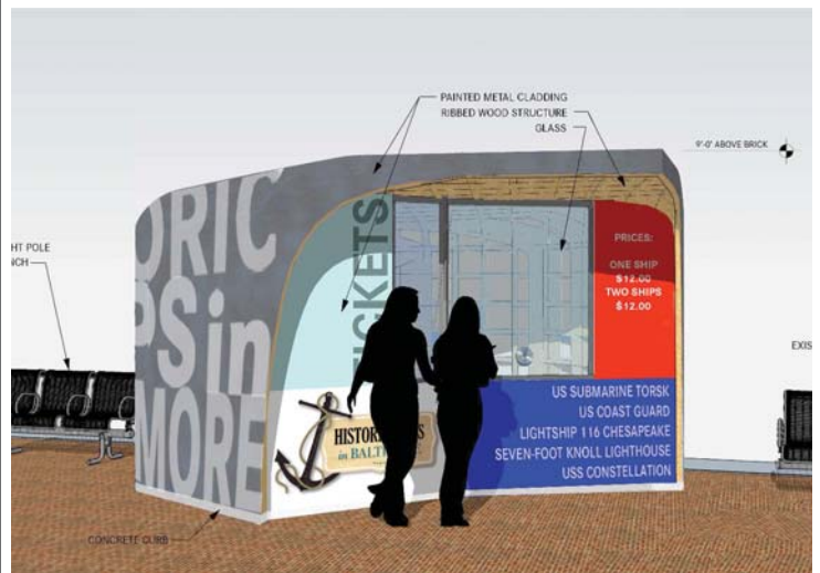
New Pier 3 Ticket Booth Looking West
