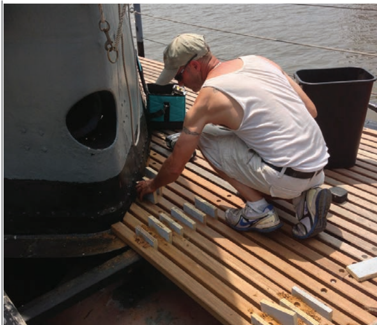
Pier 3 Site Manager Rob Howard cutting deck battens to fit the forward edge of the “sail” on board USS Torsk.
