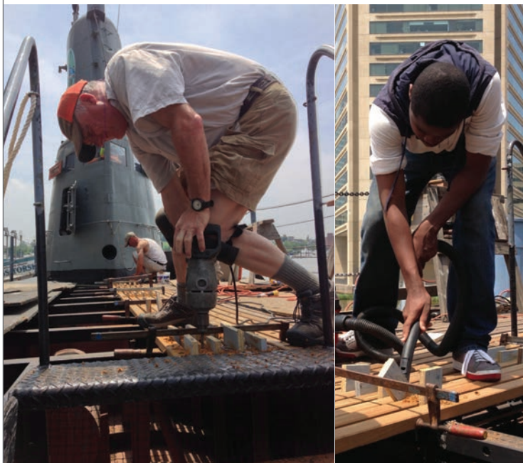
Shipwright Tim Fowler on board USS Torsk (left) drilling holes and restoration intern Xavier (right) doing some clean-up in preparation for fastening the new deck battens.
