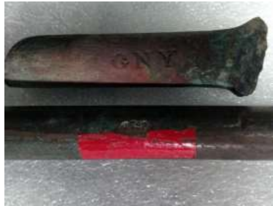
Above: "GNY" marking on a copper spike removed from a piece of CONSTELLATION's original hull planking. Below: a recently donated spike with the stamping "1797."
