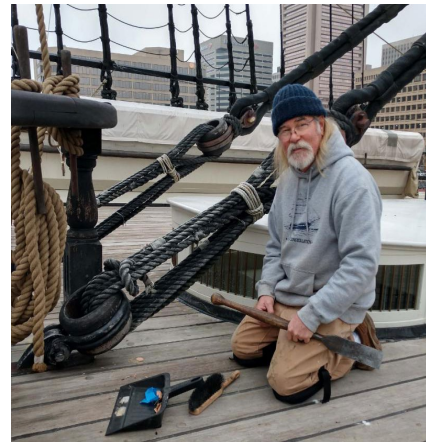
Randy Hall repairing deck caulking on USS CONSTELLATION
