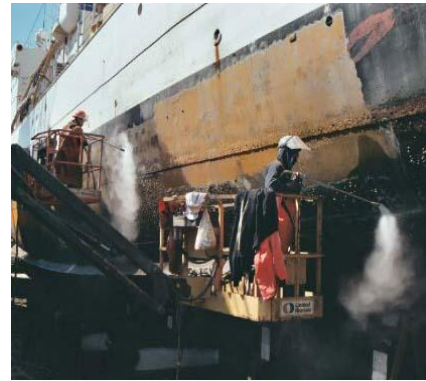
UHP hydroblasting crews clean the hull of USCGC TANEY during the ship's 2003 dry docking at the US Coast Guard YARD, Curtis Bay.
