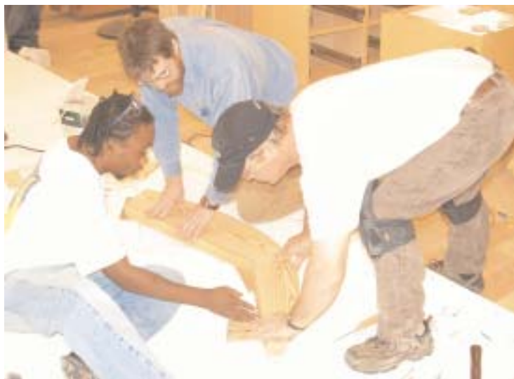
From left to right, Todd, Seth and Bruce lay out the molds on the lofting floor. Before making the molds the shipwrights drew the boats plans full size on the lofting floor to facilitate pattern making.
