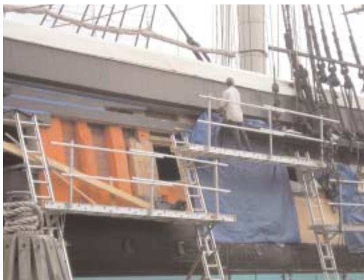
Shipwright Joan Murphy working on the hull repair.
