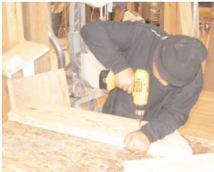
Fresh Start Student Robert drills holes in the molds prior to assembly. Once prepared, the molds will be the framework upon which the planking is laid.
