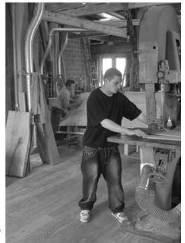
Student Justin Chilcote Uses the Ship's Saw to Shape Timbers For Constellation's Quarterboat. Photo by Marc Pettingill
