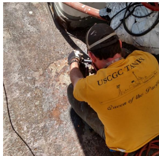
Pier 5 Manager Ryan Szimanski uses a pneumatic piston scaler to clean a portion of USCGC Taney's starboard main deck to bare metal for repair and painting.
